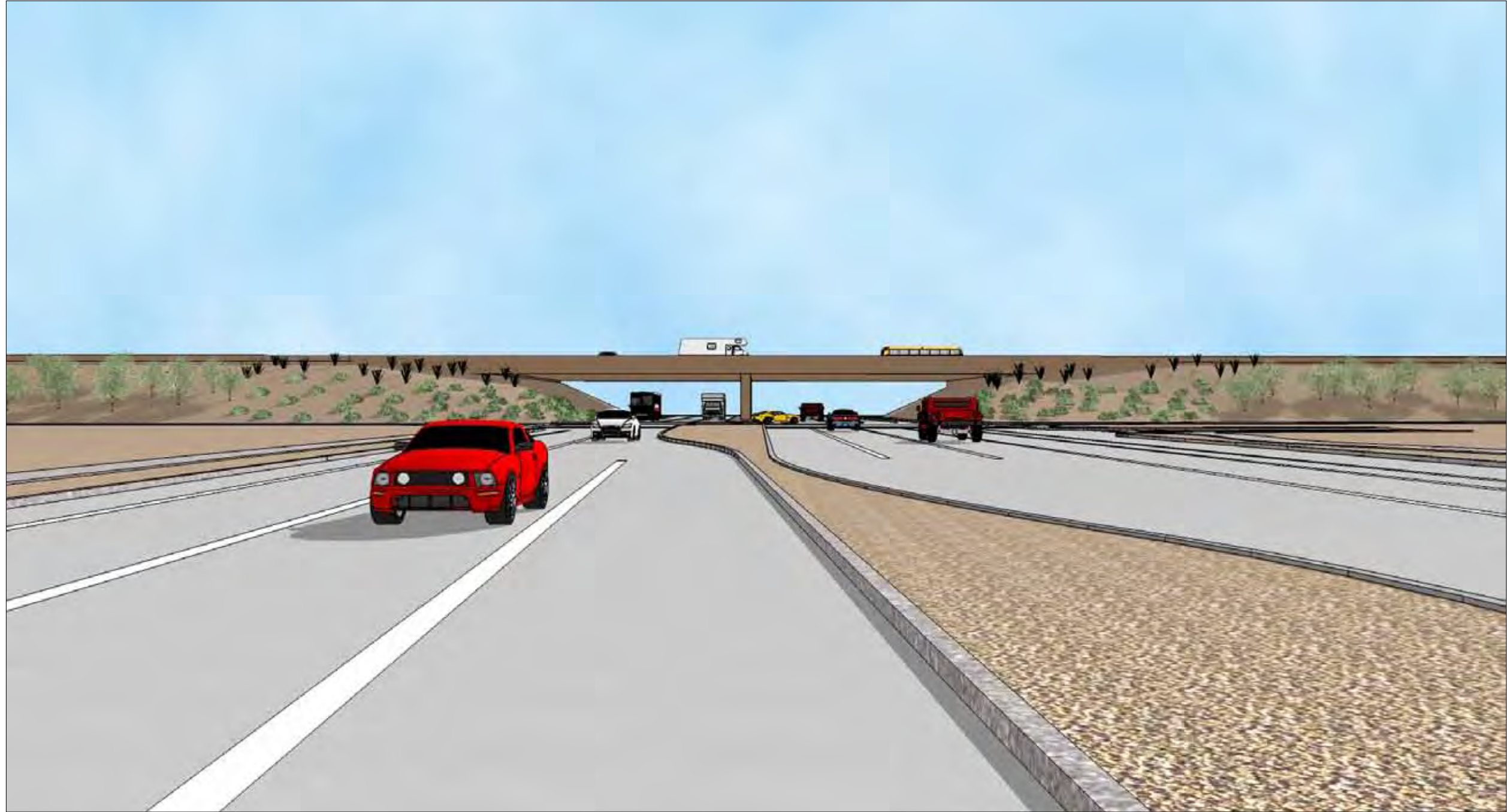
Visual simulation showing the proposed freeway from 1/4-mile north at 40th Street (looking south). The clearance from the bridge to the ground below would be approximately 17 feet. Noise walls would be added along the freeway where required.
